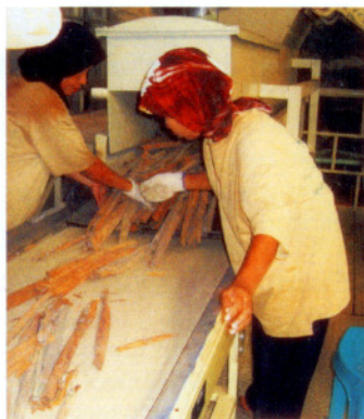
Workers arrange the quills in line as the conveyor takes the quills into the first cutter.
