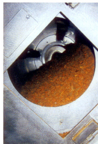
A view of the interior of the Munson rotary continuous mixer.
