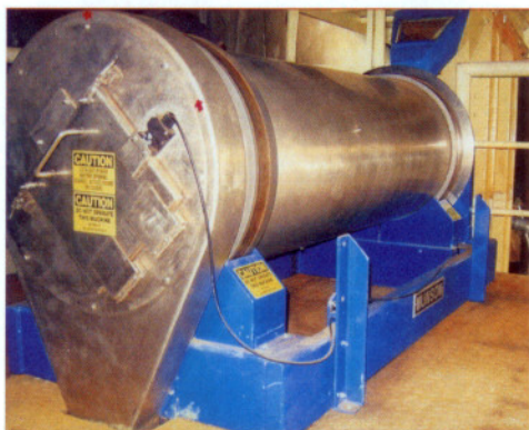
The Munson rotary continuous mixer makes a thorough blend without breaking the brittle cinnamon.
