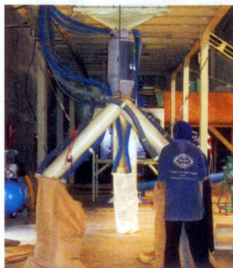
Processed cinnamon is loaded into shipping sacks through pipe magnets for last-minute removal of any ferrous metal.
