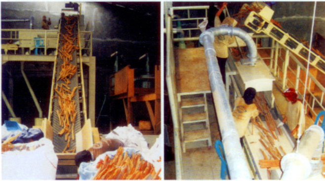
As bags of raw cinnamon quills arrive at the plant they are emptied onto a belt conveyor for processing.
