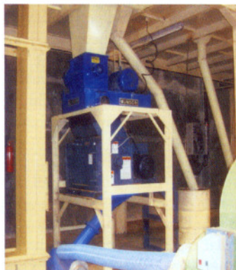
The Munson high-speed screen classifying cutter cuts the cinnamon quills into 5cm lengths.
