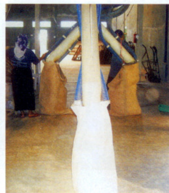
Processed cinnamon is loaded into shipping sacks through pipe magnets for last-minute removal of any ferrous metal.
